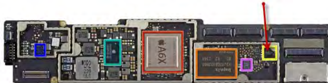
Sample iPad mini audio codec chip from teardown available at
